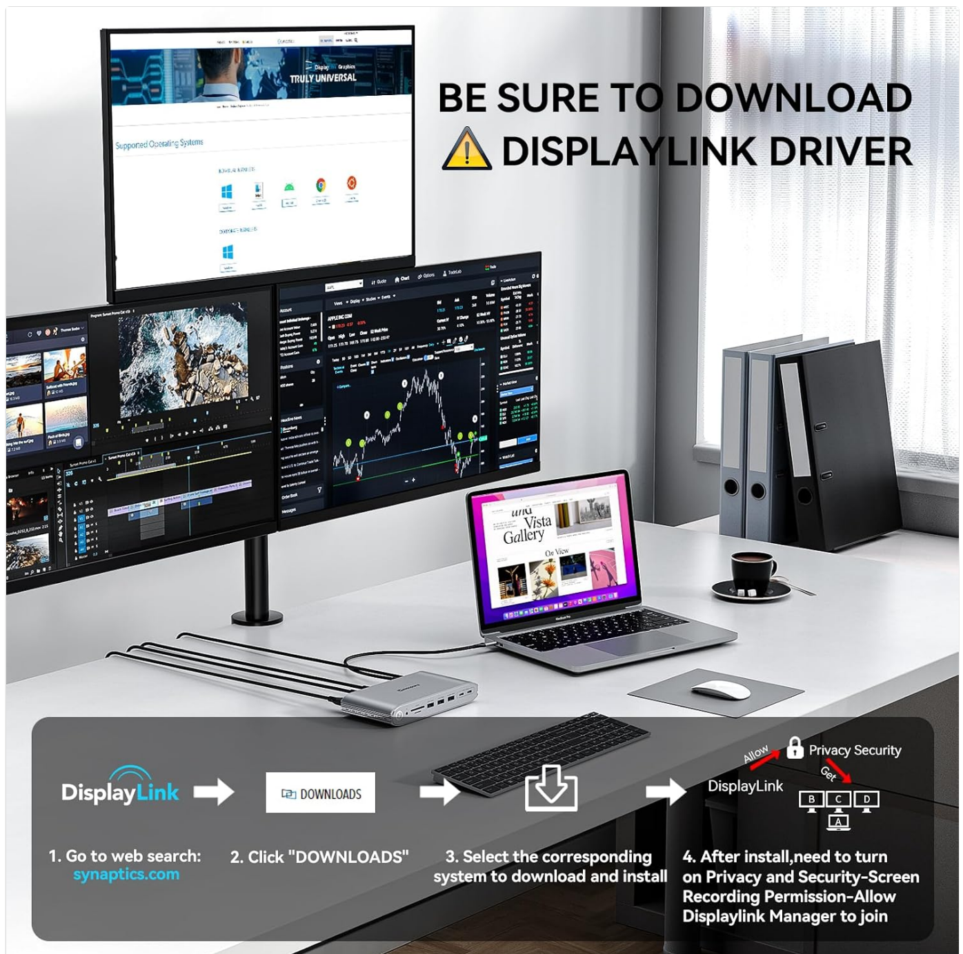
Image: Steps for installing the DisplayLink driver on your operating system.
