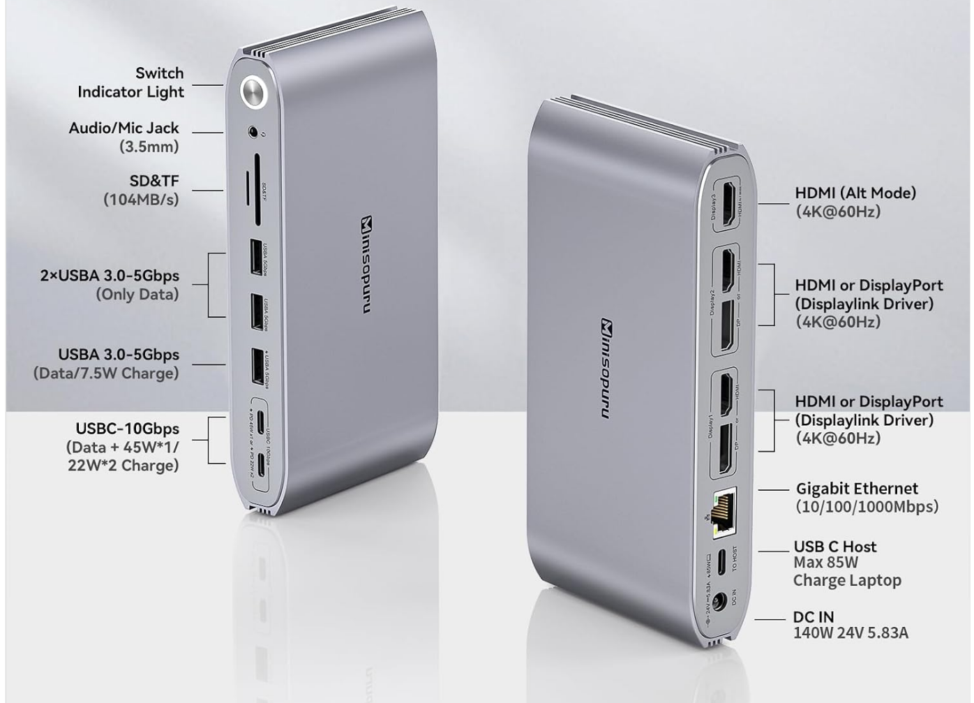
Image: Front and back view of the Minisopuru MD6950D Docking Station with all ports labeled.
