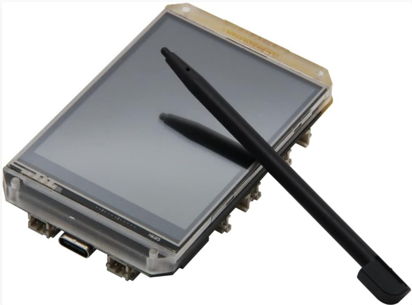
Figure 3.3: The 2.8-inch ST7789 LCD touch display module with the included resistive stylus, used for precise interaction.
