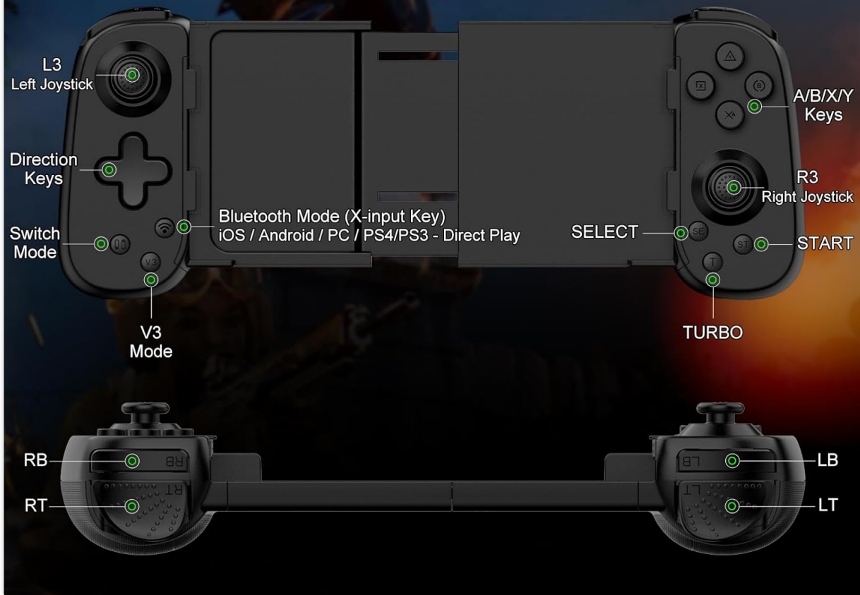
Image: A detailed diagram labeling all buttons and their functions on the Koiiko D6 controller.
