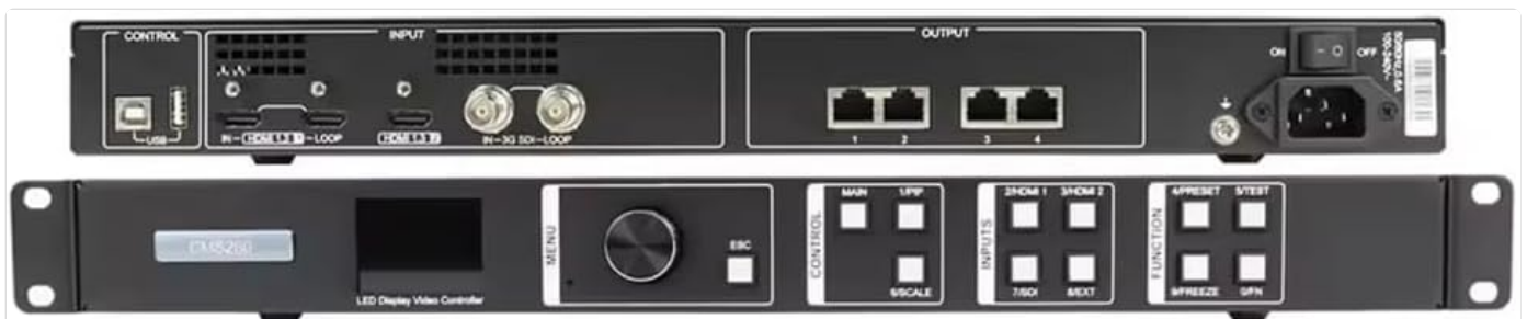
Figure 2.1: Front and Rear Panels of the CMS260 LED Video Controller. The top image shows the rear panel with control, input (USB, HDMI, SDI), and output (Ethernet) ports. The bottom image displays the front panel with navigation buttons, an LCD screen, and function keys for control and input selection.
