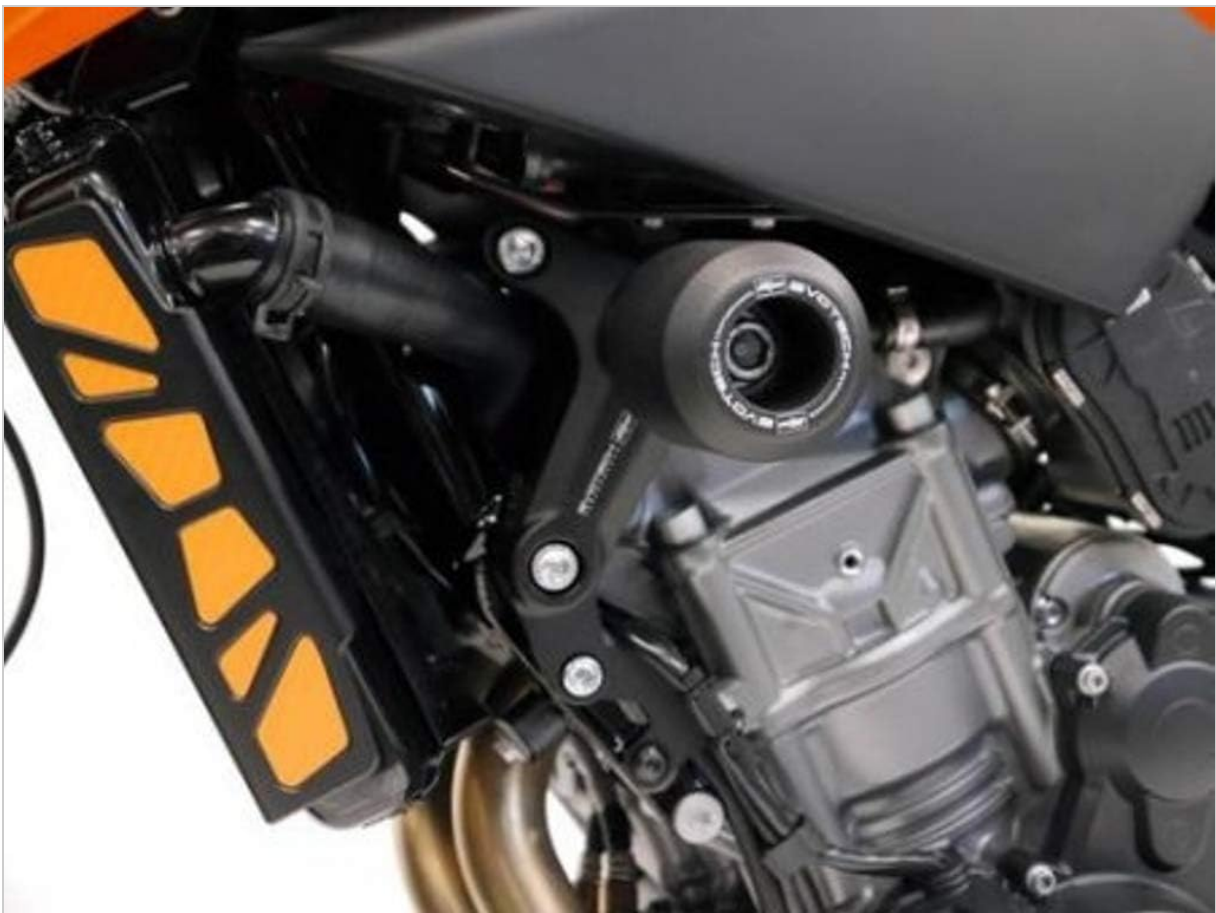
Figure 4.2: Wider view of the crash protection installed on a KTM motorcycle, showing overall fitment.
