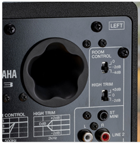
Image: Close-up view of the 'ROOM CONTROL' and 'HIGH TRIM' switches on the rear panel, showing their adjustable settings.
