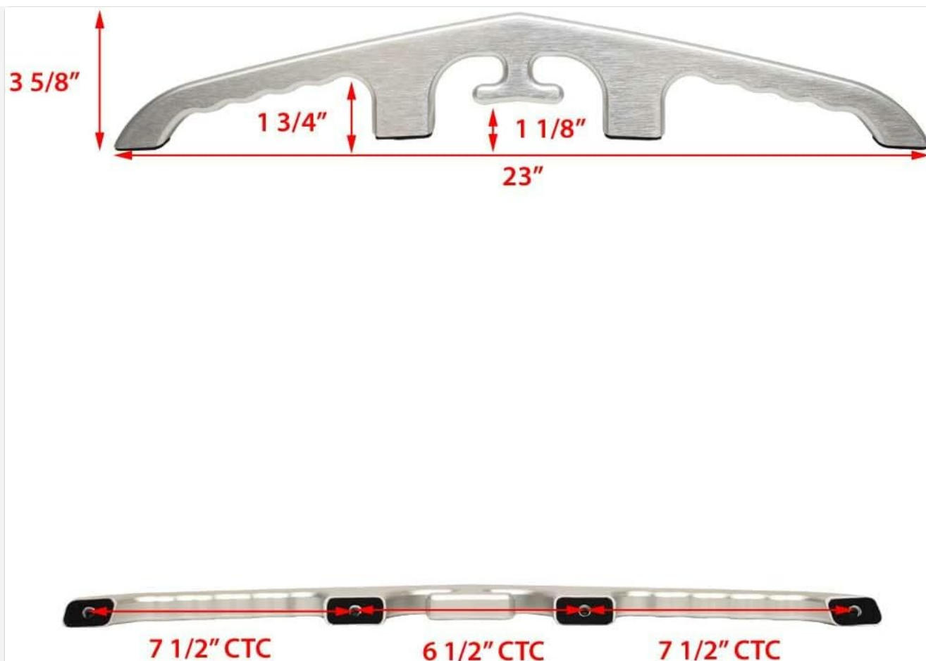
Figure 4: Dimensional drawing of the grab rail, showing overall width and height, and mounting hole spacing.
