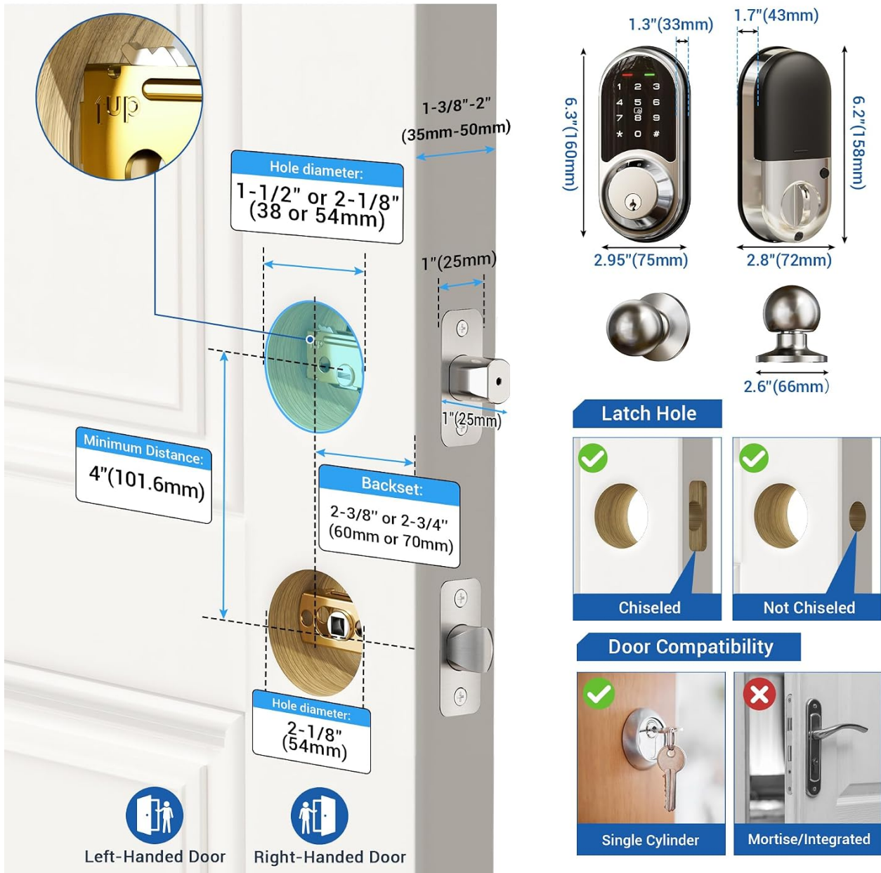
Image: Detailed diagram illustrating the necessary door dimensions and compatibility requirements for installing the Veise smart lock.
