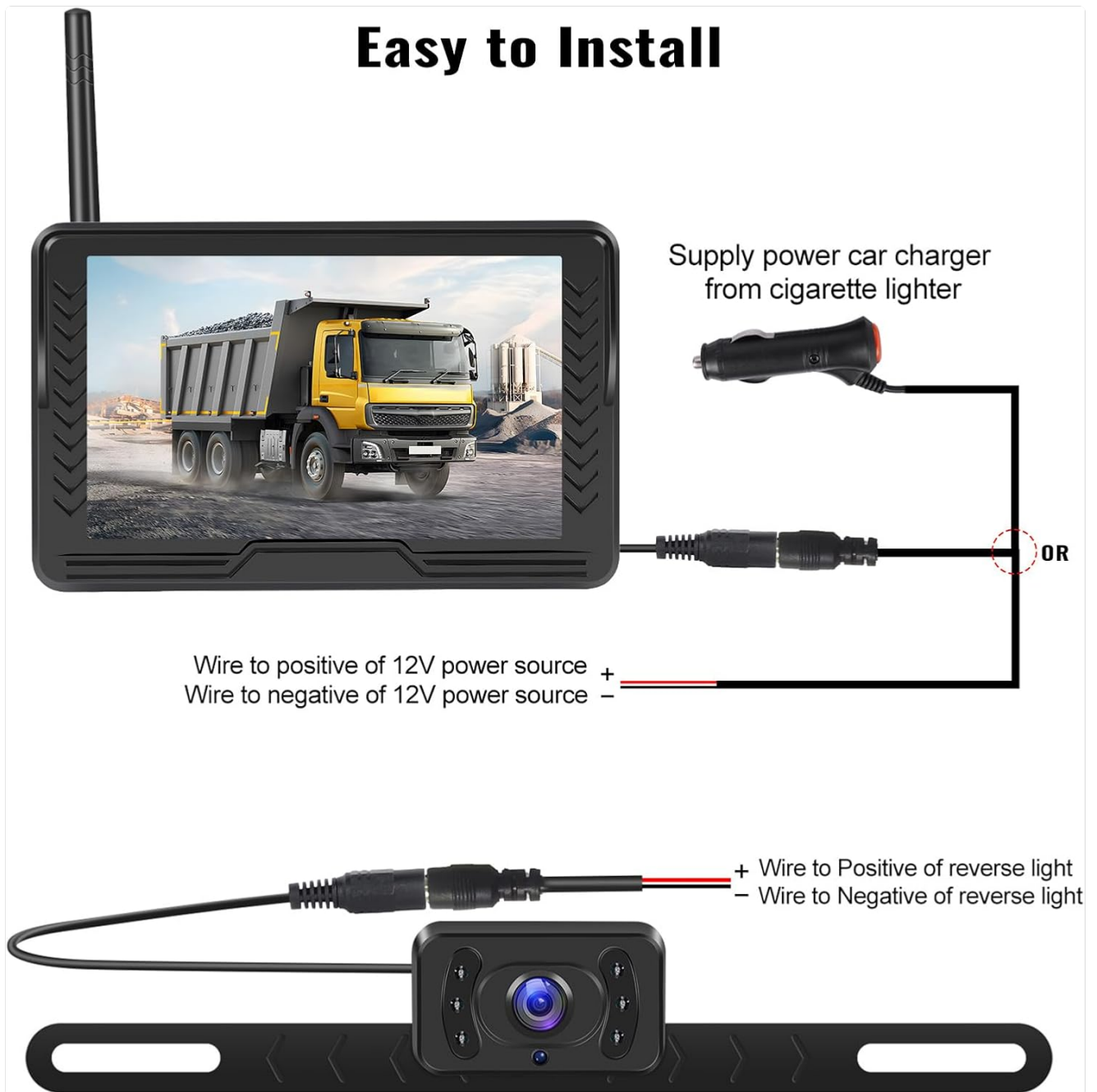
Figure 4: Wiring diagram for monitor and camera.
