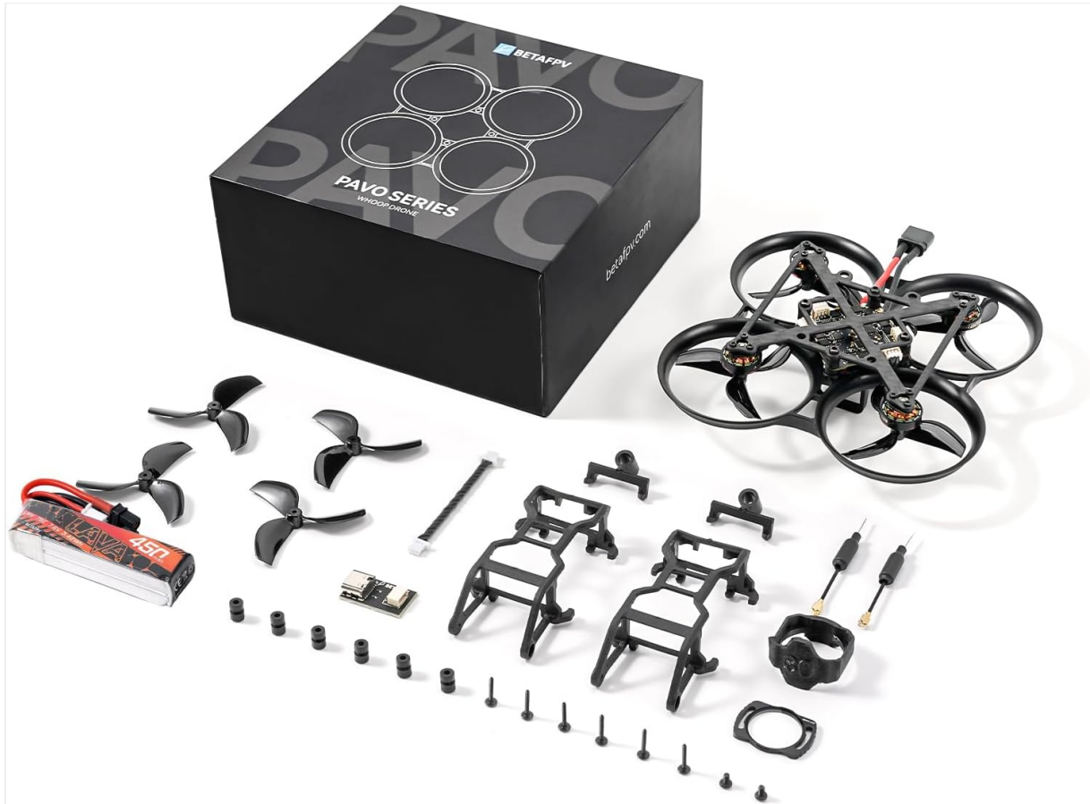
Image: All components included in the BETA FPV Pavo Pico package.
