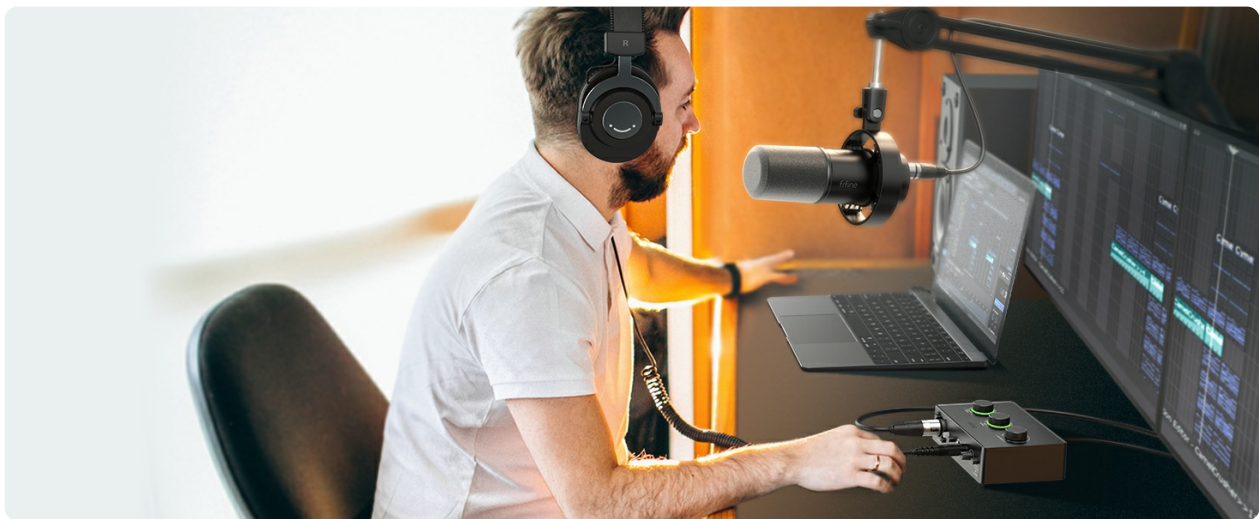
Figure 14: A condenser microphone connected to the audio mixer, utilizing the 48V phantom power feature.
