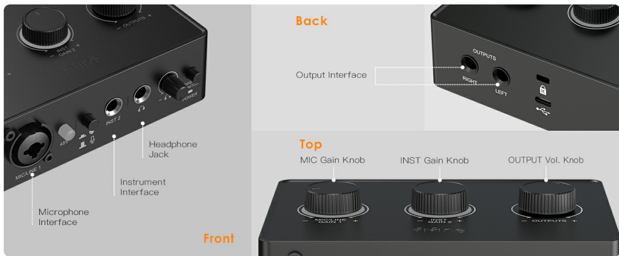
Figure 16: Dedicated volume knobs for both output and headphones, allowing precise control over playback levels.
