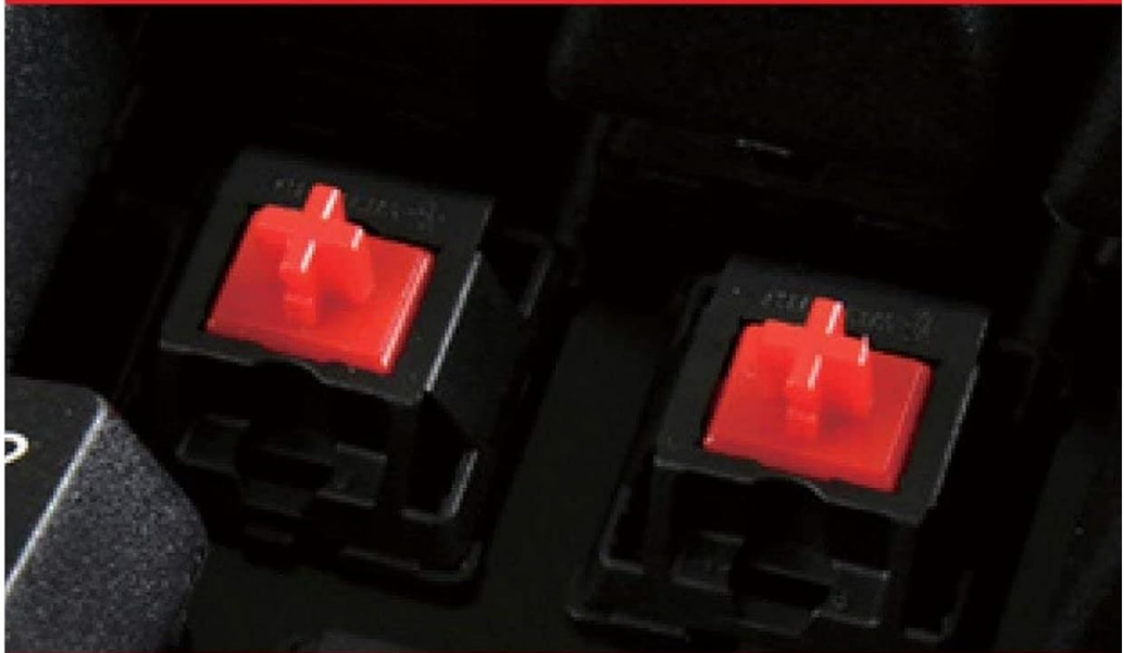
Figure 7.1: Cherry MX Red Switches. This image provides a close-up view of the Cherry MX Red mechanical switches, which are linear and known for their smooth, consistent keystrokes without a tactile bump or audible click.
