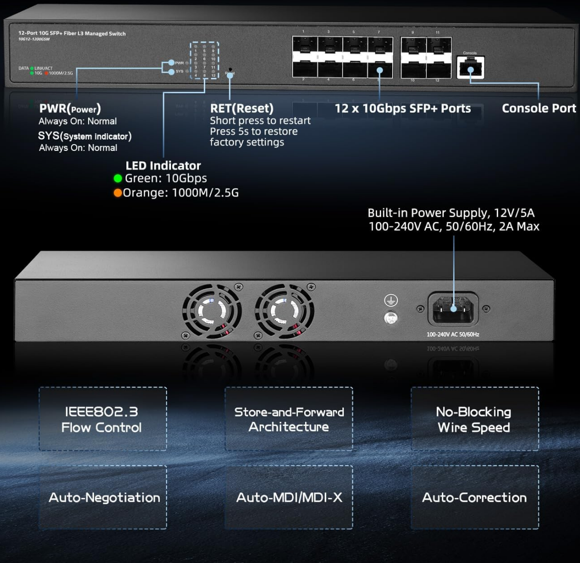
Image 4.1: Detailed view of the 12-Port 10G SFP+ Optical Ethernet Switch, showing the PWR (Power) and SYS (System) LED indicators, RET (Reset) button, 12x 10Gbps SFP+ Ports, and Console Port. The image also highlights the built-in power supply and various network standards supported.
