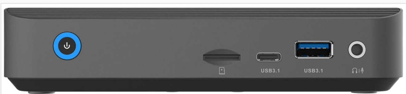
Image 3.1: Front view of the ZOTAC ZBOX-CI343-BE, showing the power button, USB 3.1 ports, USB-C port, SD card slot, and audio jack.
