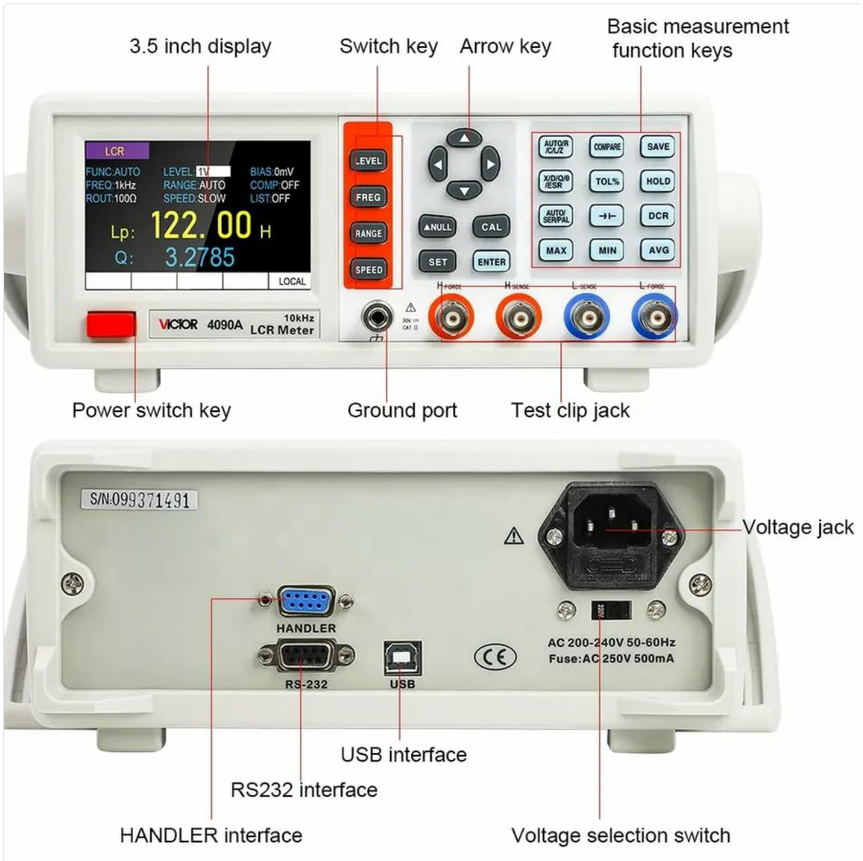
Figure 3: Rear panel showing the voltage jack, voltage selection switch, USB interface, RS232 interface, and HANDLER interface.
