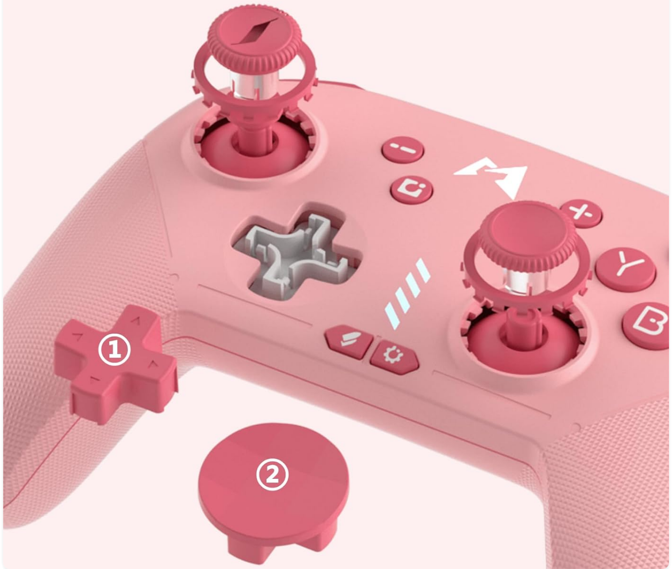
Image: Close-up view of the interchangeable D-pad mechanism and the two D-pad styles.
