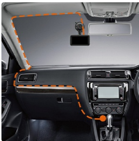
Image: An overhead view diagram of a car interior, showing the suggested path for routing the dash cam's power and rear camera cables discreetly along the dashboard and A-pillar.
