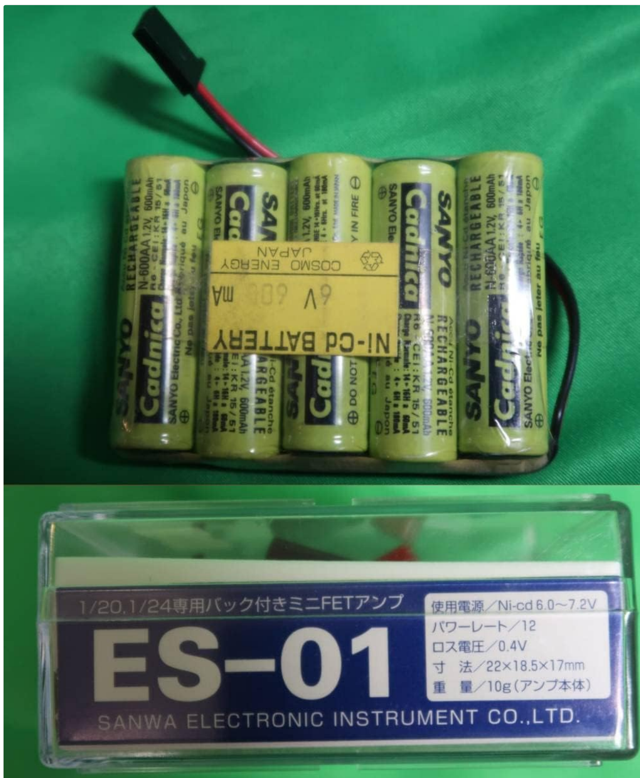
Figure 3.7: Close-up of the Sanyo Cadnica 6V 600mAh Ni-Cd battery pack and Sanwa ES-01 mini FET amplifier. A detailed view of the Sanyo Cadnica 6V 600mAh Ni-Cd battery pack and the Sanwa ES-01 mini FET amplifier, showing their labels and specifications.
