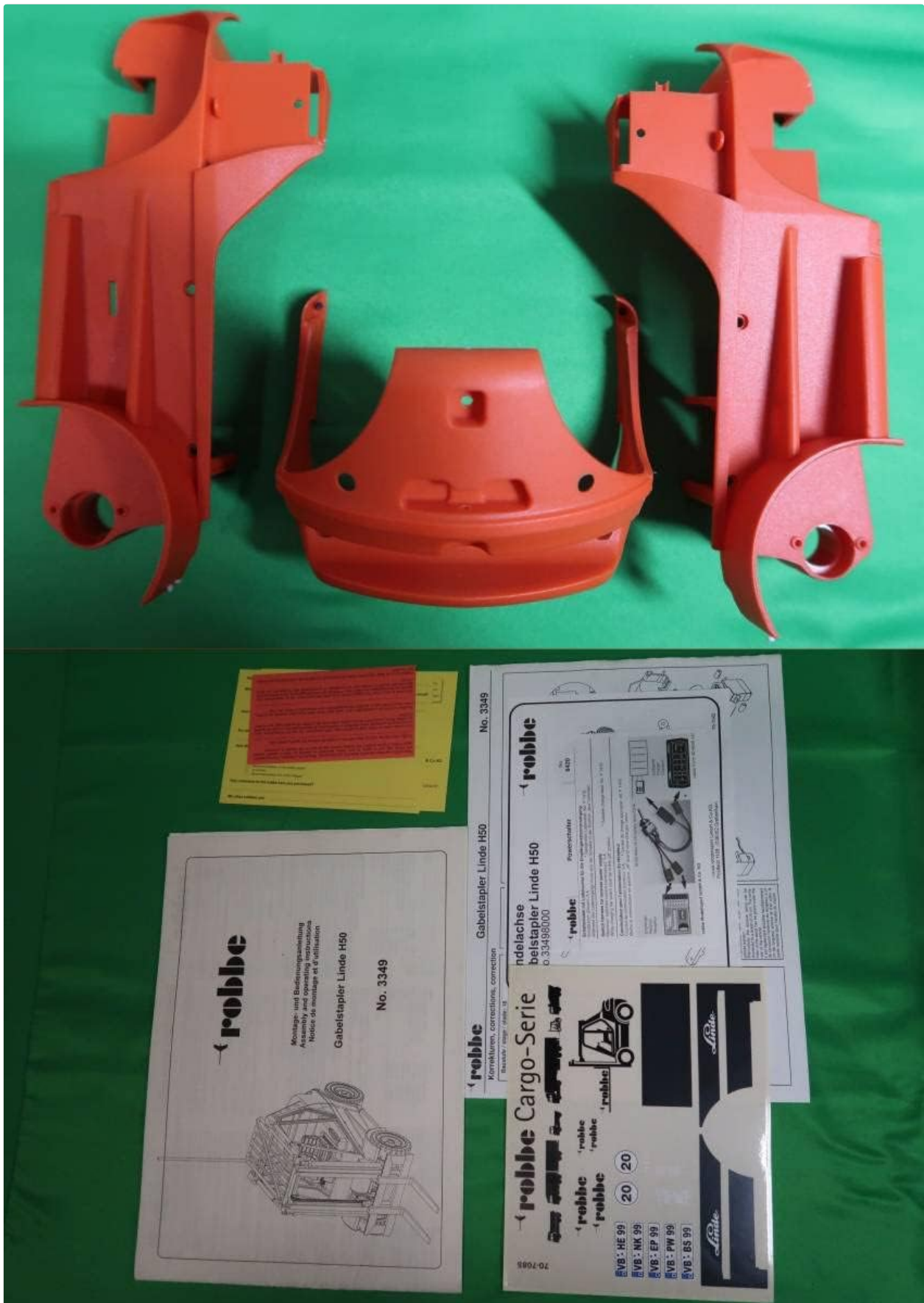
Figure 3.9: Main body shell components and instruction manuals for the Robbe 1/16 Linde H50 RC Forklift. This image shows the main orange plastic body shell components of the forklift, along with the primary instruction manual for the Linde H50 model and additional documentation for accessories and parts.
