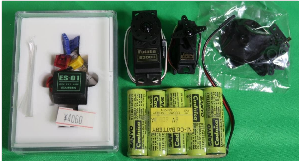
Figure 3.6: Electronic components for the RC forklift, including Futaba servos and a Sanyo Cadnica battery pack. Key electronic components are displayed, including two Futaba S3003 servos, a Sanwa ES-01 mini FET amplifier, and a Sanyo Cadnica 6V 600mAh Ni-Cd rechargeable battery pack, essential for the forklift's operation.
