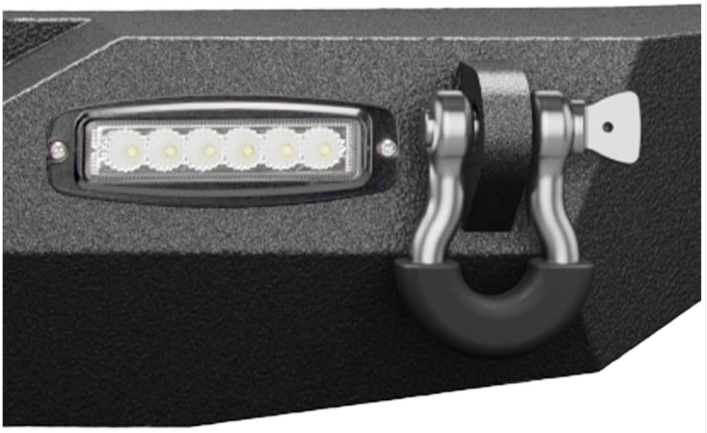
Figure 6: Detail of D-ring shackle mount and LED light.
