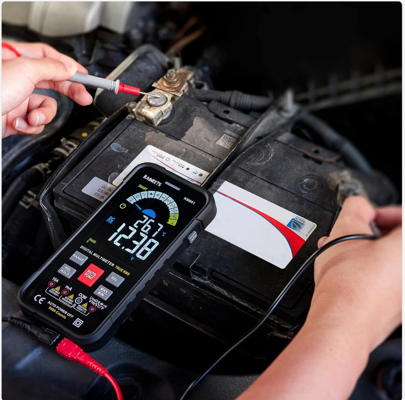
Figure 7: The multimeter being used to measure voltage on a car battery.
