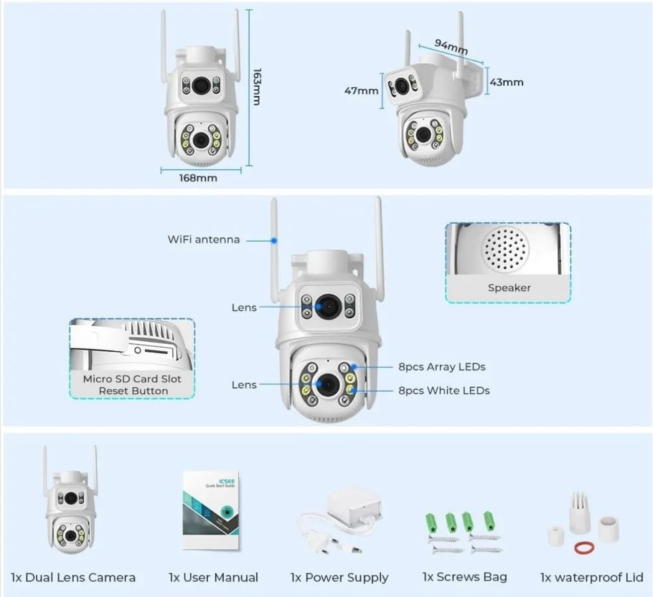
Figure 2.1: Product Components and Dimensions. This image illustrates the physical layout of the camera, highlighting key parts such as the dual lenses, WiFi antennas, speaker, and the location of the Micro SD card slot and reset button. Dimensions are provided for overall height (163mm), width (168mm), and top section measurements (94mm, 47mm, 43mm).
