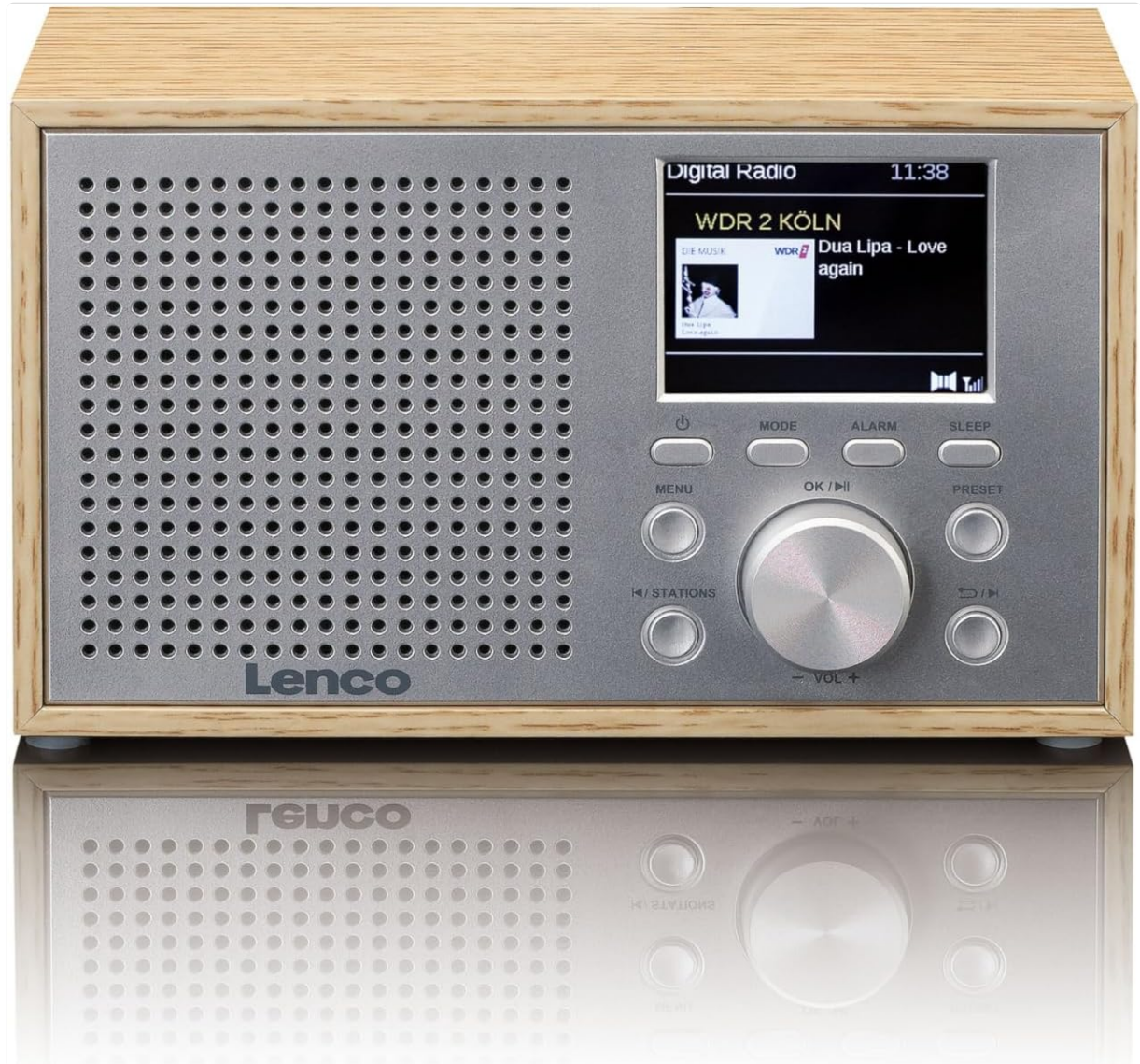
Image: Front view of the Lenco DAR-017WH radio, showing the speaker grille on the left, the 2.4-inch TFT LCD display on the right, and various control buttons and a rotary knob below the display. The casing is light wood.
