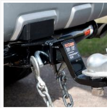
Image: A close-up view of the standard 2-inch hitch receiver, ready for a ball mount or other towing accessories.
