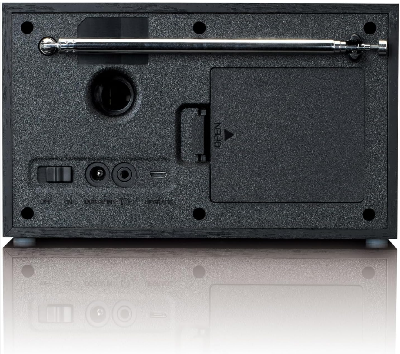
Figure 2.3: Back View. This image illustrates the rear panel of the Lenco DAR-017 DAB+ Radio. It features an ON/OFF switch, DC 5V IN port, a 3.5mm AUX input/headphone output, a micro-USB port (likely for firmware upgrades), and a battery compartment cover labeled "OPEN". The telescopic antenna base is also visible at the top.
