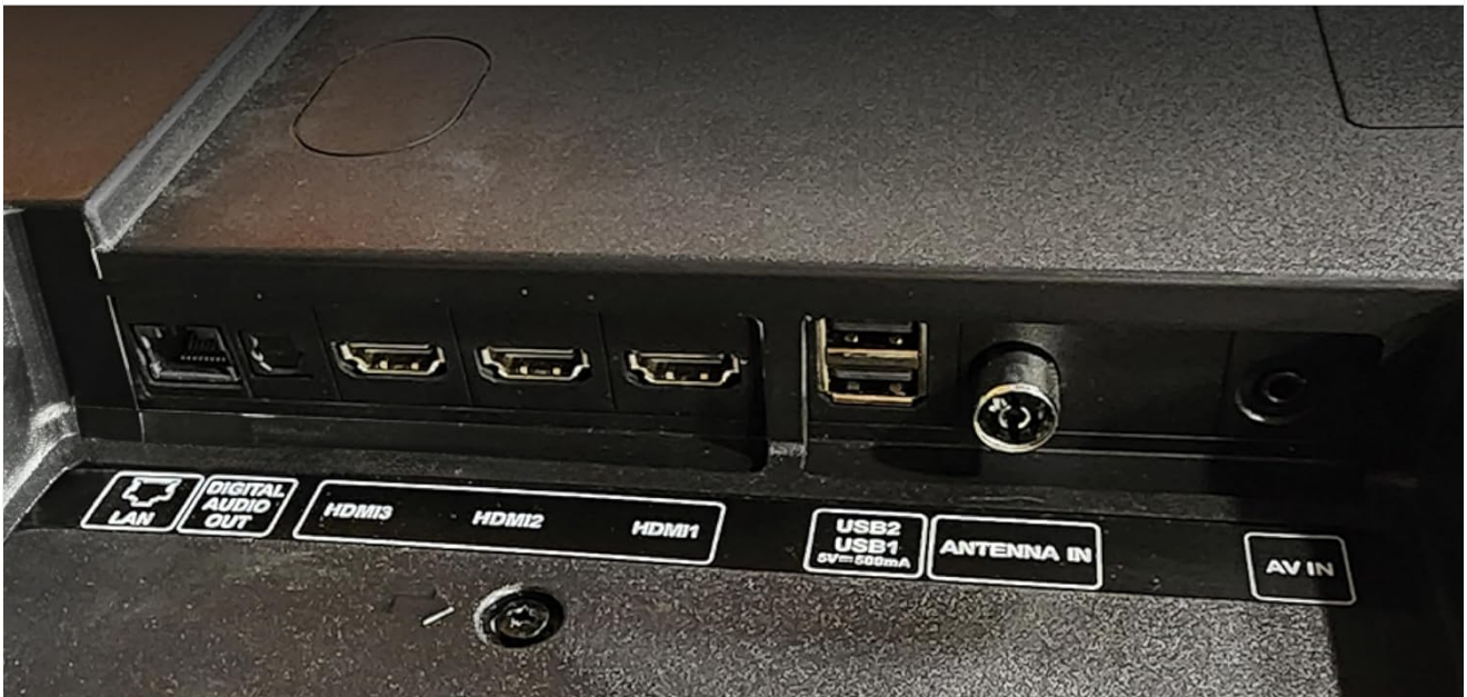
Figure 4.3: Detailed view of the TV's connectivity ports including LAN, HDMI, USB, Antenna In, and AV In.
