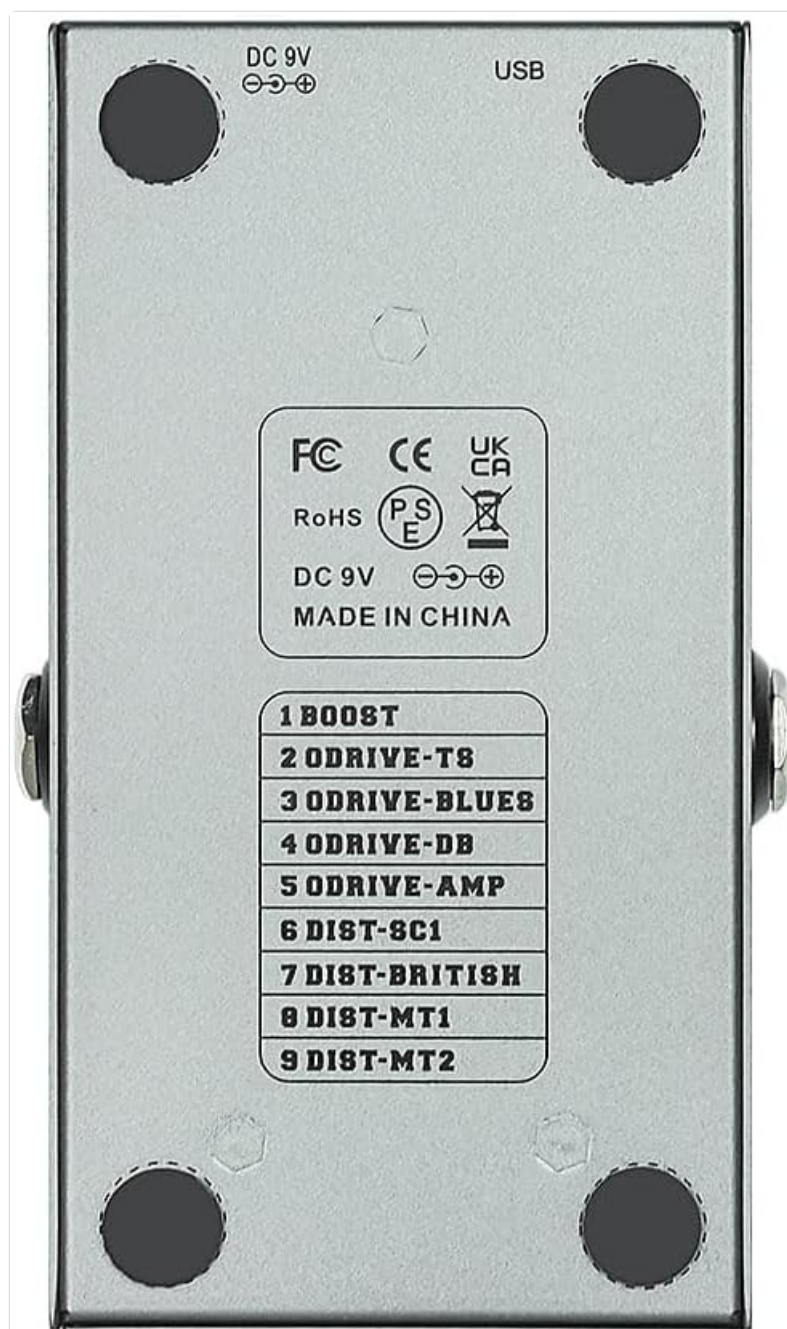
Figure 2: Rear view of the Mini EFX pedal, showing the DC 9V power input and regulatory compliance markings.
