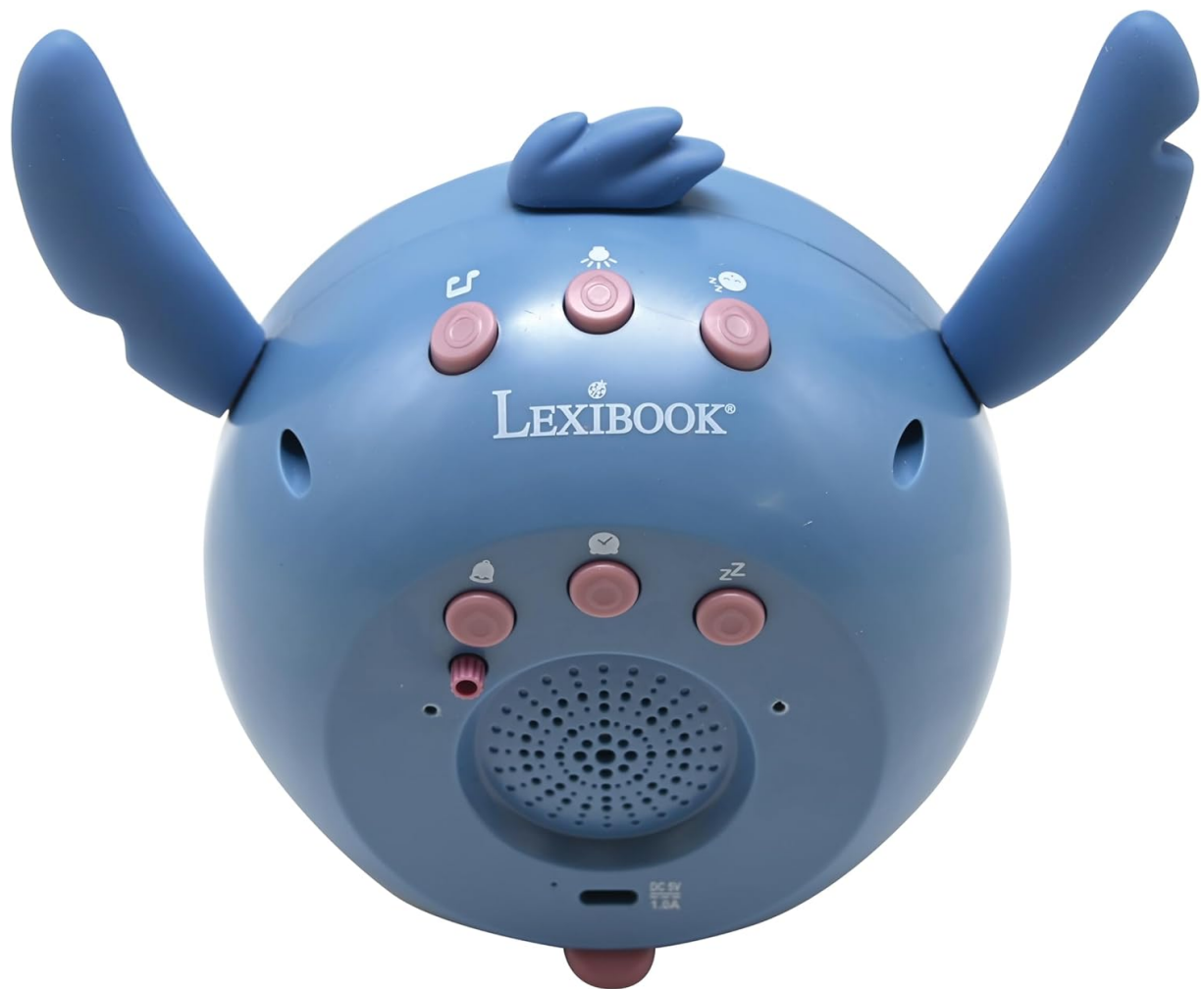
Image: Rear view of the Lexibook Disney Stitch Night Companion, showing the USB-C port, speaker, and control buttons.
