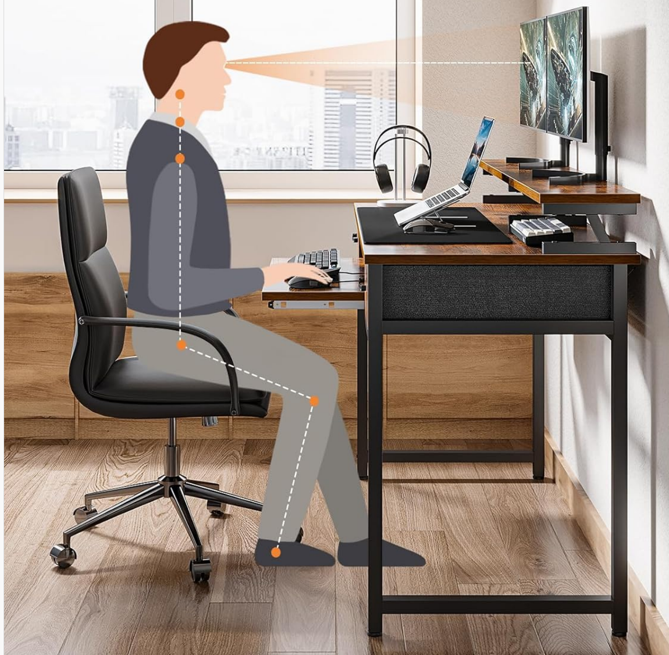
Figure 5.2: An illustration demonstrating the ideal ergonomic sitting posture at the desk, emphasizing monitor height and keyboard placement to reduce strain.
