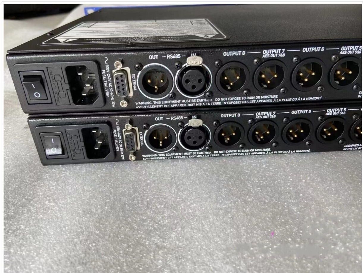
Figure 4.1: Rear panel connections of the XTA DP448 Audio Processor. This image displays the power input, RS485 control ports, and multiple audio output connectors, including AES/EBU digital and analog XLR outputs, essential for integrating the processor into an audio system.
