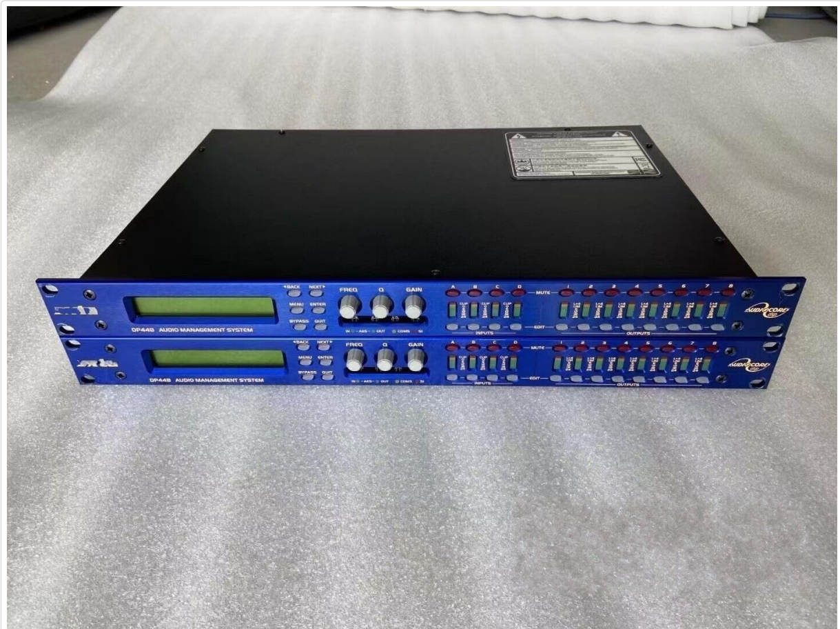
Figure 5.1: Front panel display and navigation controls. This detailed view highlights the LCD screen, which displays operational parameters and menu options, along with the 'BACK', 'NEXT', 'MENU', 'ENTER', 'BYPASS', and 'QUIT' buttons used for navigating the system's interface.
