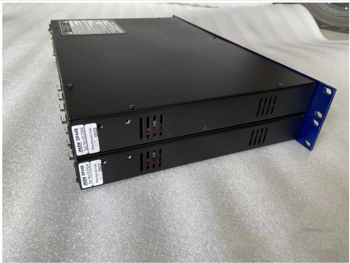
Figure 6.1: Side view showing ventilation grilles. This image illustrates the side panel of the XTA DP448, highlighting the ventilation grilles which are crucial for dissipating heat and maintaining optimal operating temperature for the internal components.
