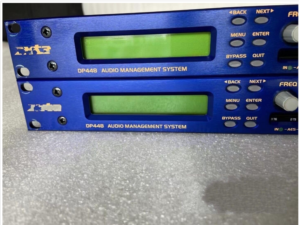
Figure 4.2: Front view of the XTA DP448 Audio Processor. This image shows the overall design, including the bright blue chassis, the clear green LCD screens for status and menu navigation, and the array of control buttons and rotary knobs used for system configuration and real-time adjustments.
