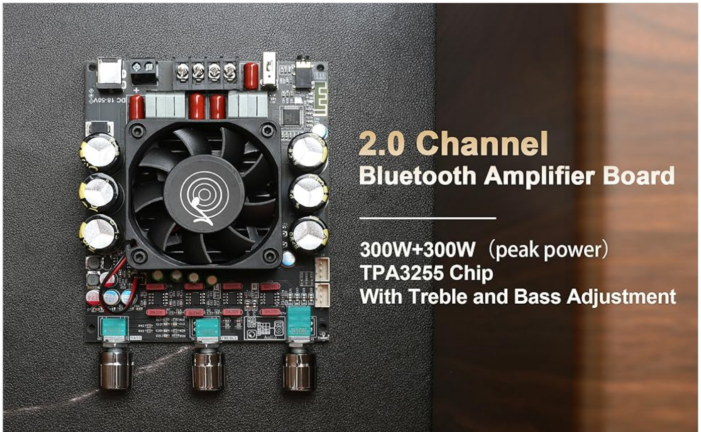
Figure 2.2: The ZK-3002T amplifier board highlighting its 300W+300W peak power and TPA3255 chip.
