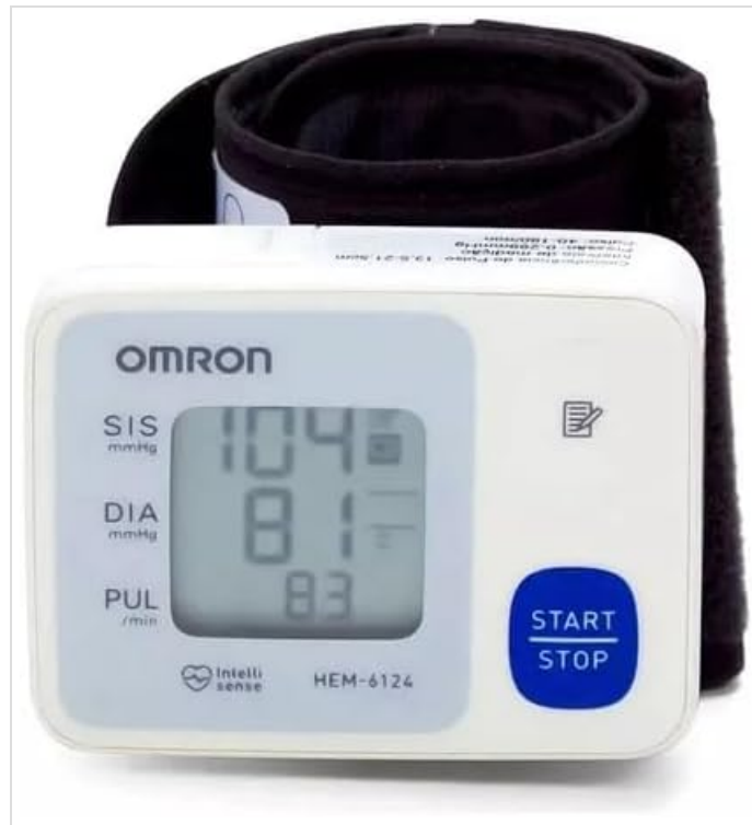
Figure 3: Displaying measurement results. This image shows the Omron HEM-6124 monitor with its digital display active, showing typical blood pressure readings (SYS and DIA) and pulse rate after a measurement has been taken.
