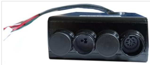
Figure 2: Close-up view of the connection ports on the FR Emomo Heat and Massage Junction Box, illustrating the different types of input/output sockets.
