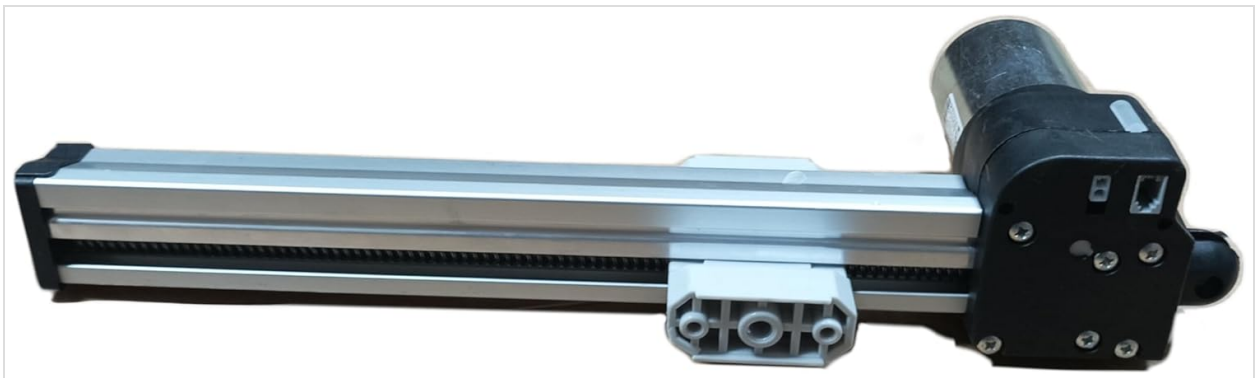
Figure 3.3: Extended view of the FR Ciar Linear Actuator Motor, showing the full travel length.
