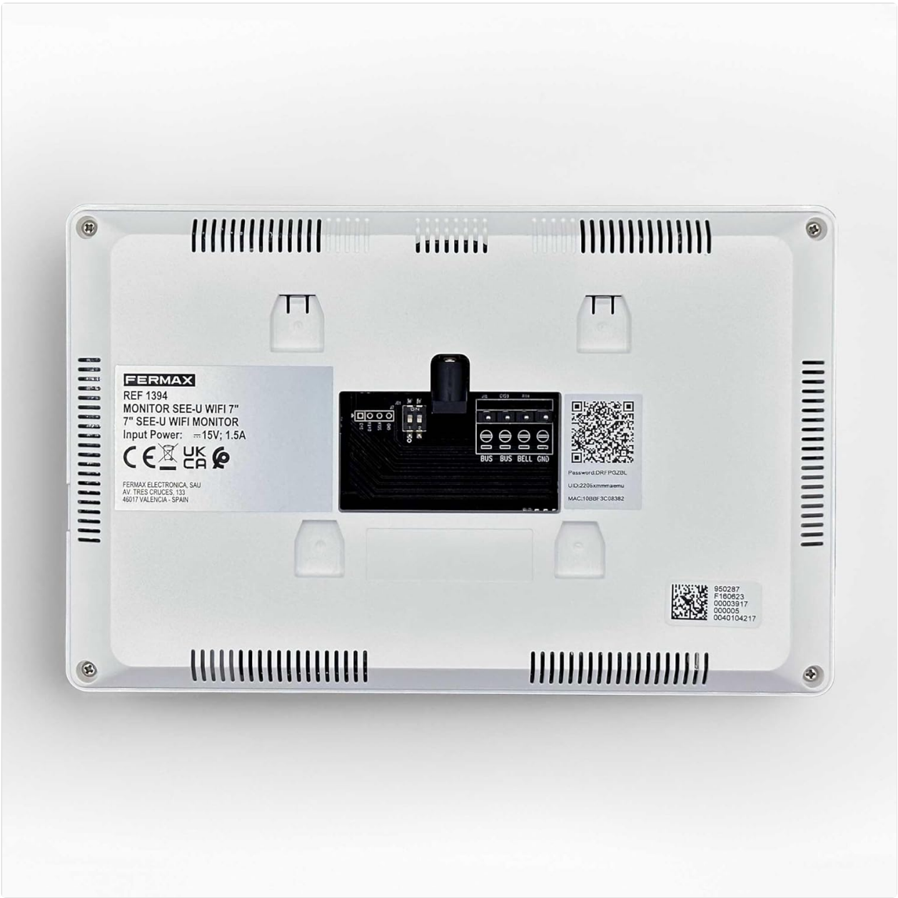
Figure 4.4.1: Back of the Fermax SEE-U monitor showing the terminal block for BUS connections and micro-switches. The diagram indicates the correct micro-switch configuration for the furthest monitor.
