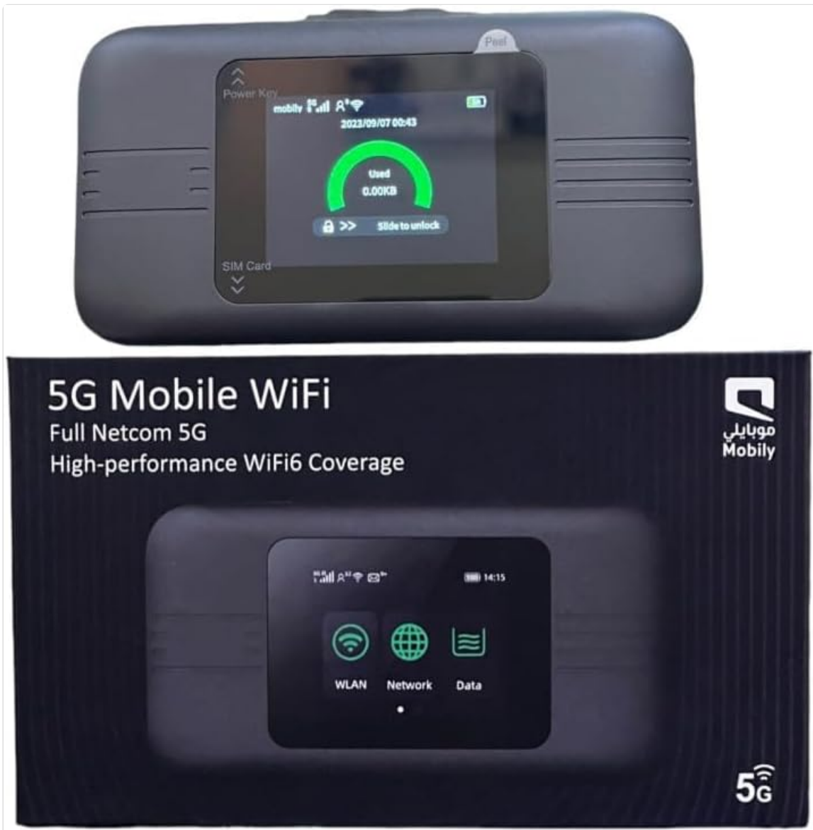
Image: The touchscreen display of the SRT875 router showing current network signal strength, battery level, time, and data usage (0.00KB used).
