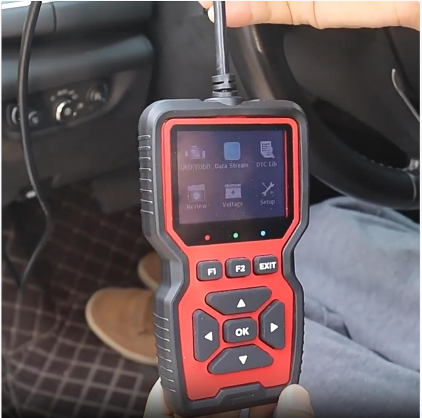
Image 3.1: The diagnostic tool being connected to the vehicle's OBD-II port, typically located under the dashboard.
