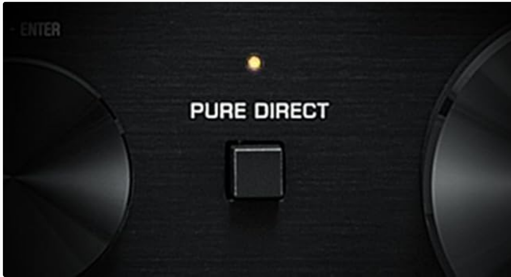
Figure 3.2: The Pure Direct button for bypassing tone controls.
