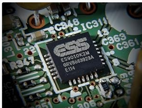
Figure 6.1: The ESS SABRE ES9010K2M DAC chip, providing superior signal-to-noise performance.
