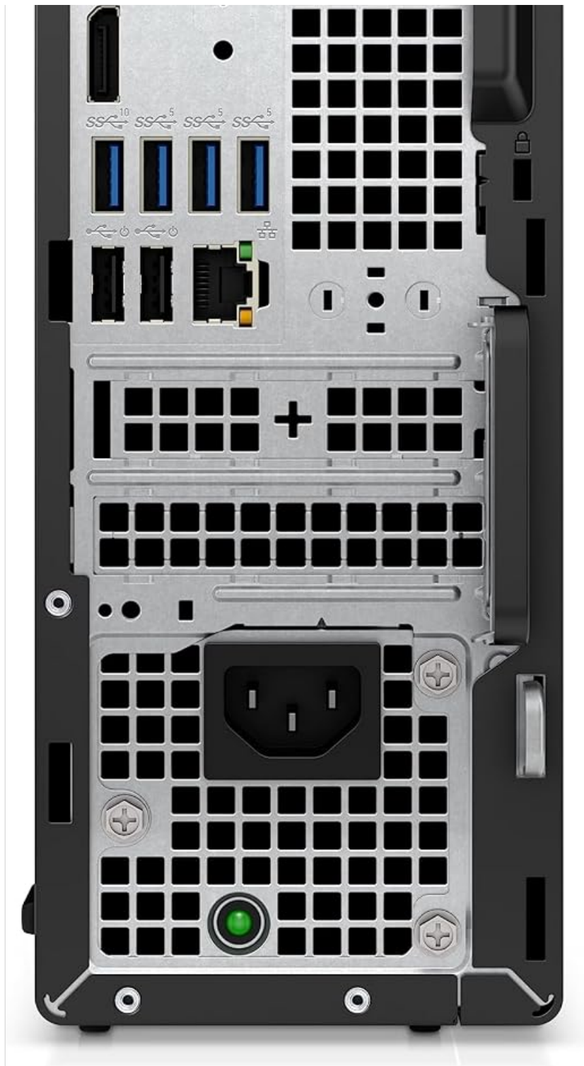
Image: Rear view of the Dell OptiPlex 7000 7020 Plus Micro PC, showing various ports including DisplayPort, USB, Ethernet, and power input.
