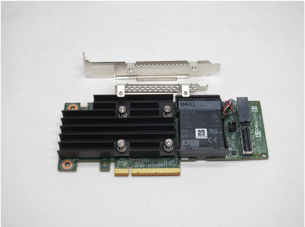
Figure 1: Front view of the Epoch DELL PERC H755 RAID Adapter, showing the heatsink and included full-height bracket. This image displays the primary components of the adapter, including the PCIe connector and various chips.
