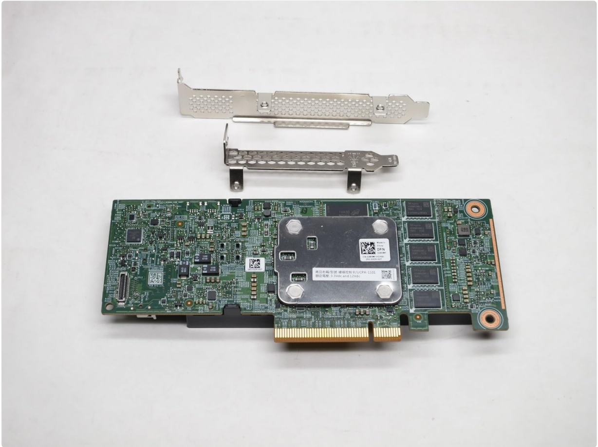
Figure 2: Rear view of the Epoch DELL PERC H755 RAID Adapter, illustrating the reverse side of the PCB with additional components and mounting points. The low-profile bracket is also visible above the card.
