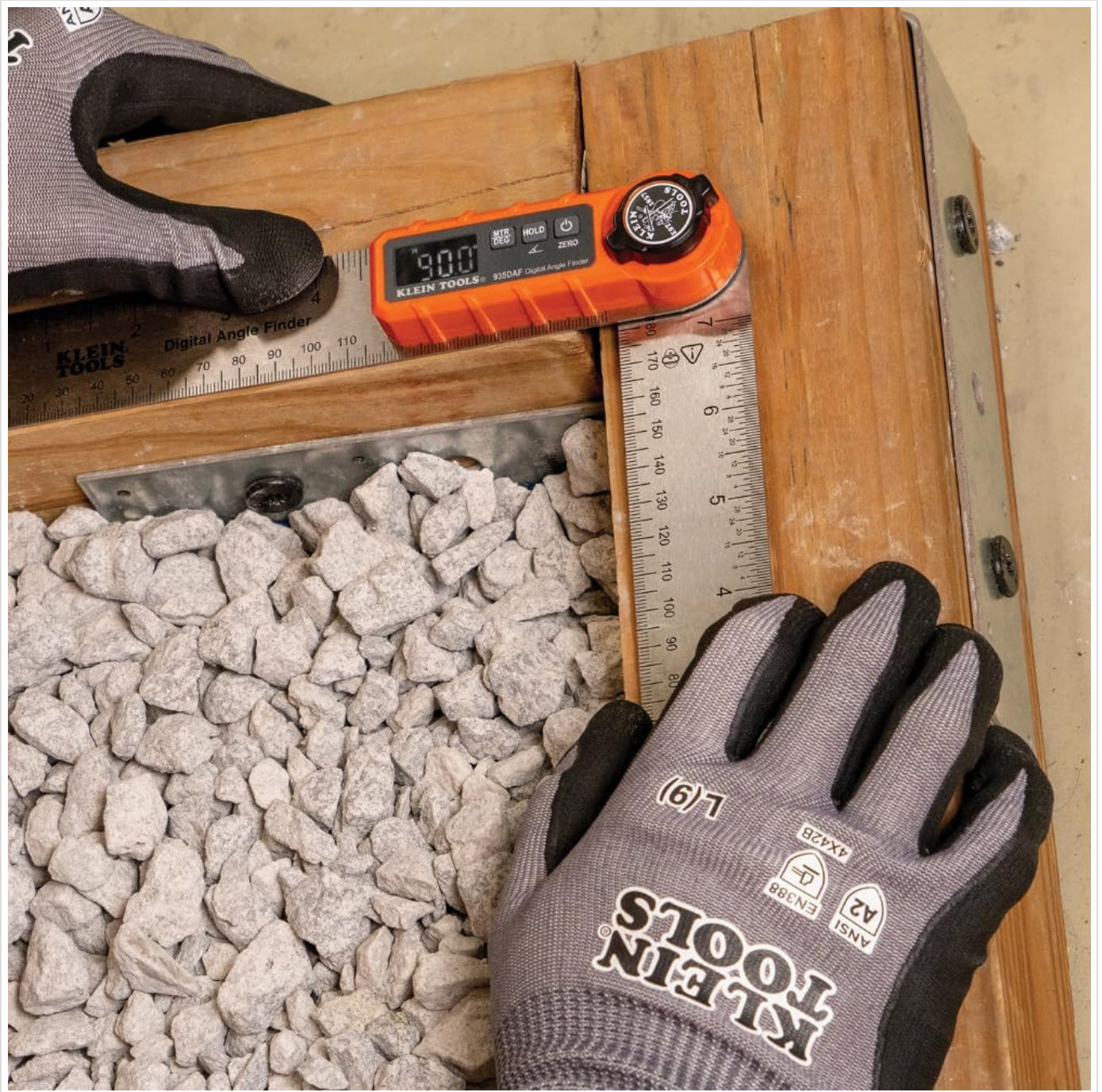
Image: The digital angle finder positioned to measure a 90-degree angle on a wooden structure, displaying "90.0" on its screen.
