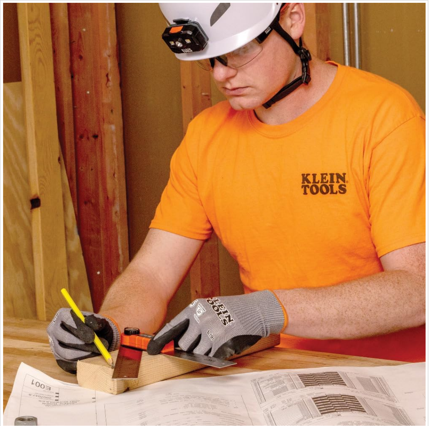
Image: A user wearing work gloves uses the digital angle finder to measure and mark an angle on a piece of wood with a yellow pencil.
