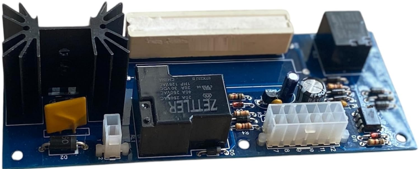
Figure 1: Overview of the 238877 Motor Feed Replacement Control Board, highlighting the 12-pin connector for easy identification during installation.
