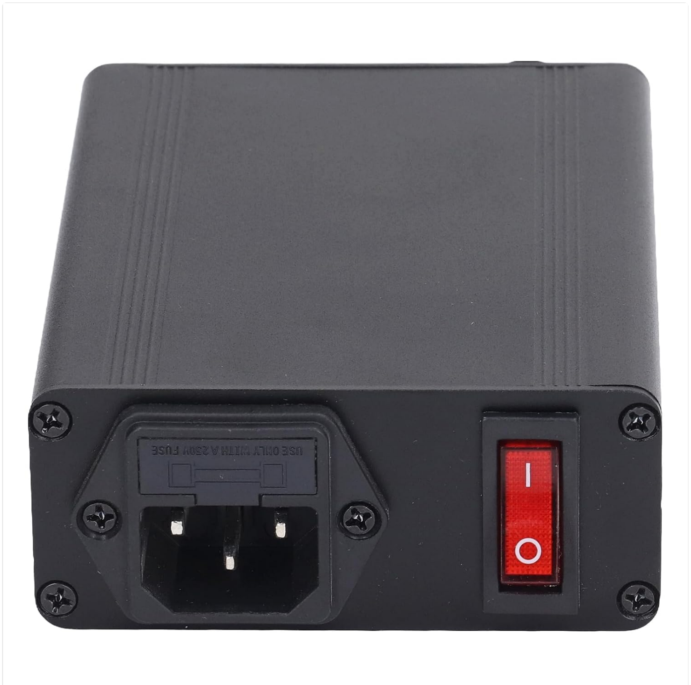
Figure 2: Rear view of the controller, illustrating the power input and main power switch.
