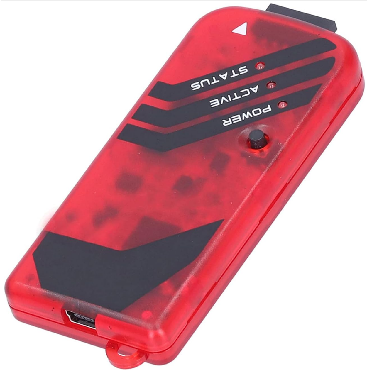
Image 3.1: The PICKit3 programmer with its USB and ICSP connection ports visible.
