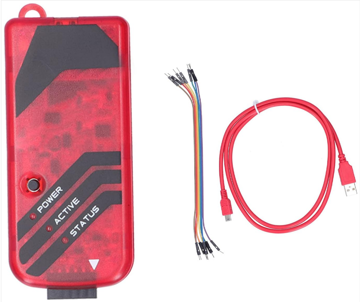
Image 2.1: The PICKit3 programmer unit, USB cable, and ICSP connection cable.
