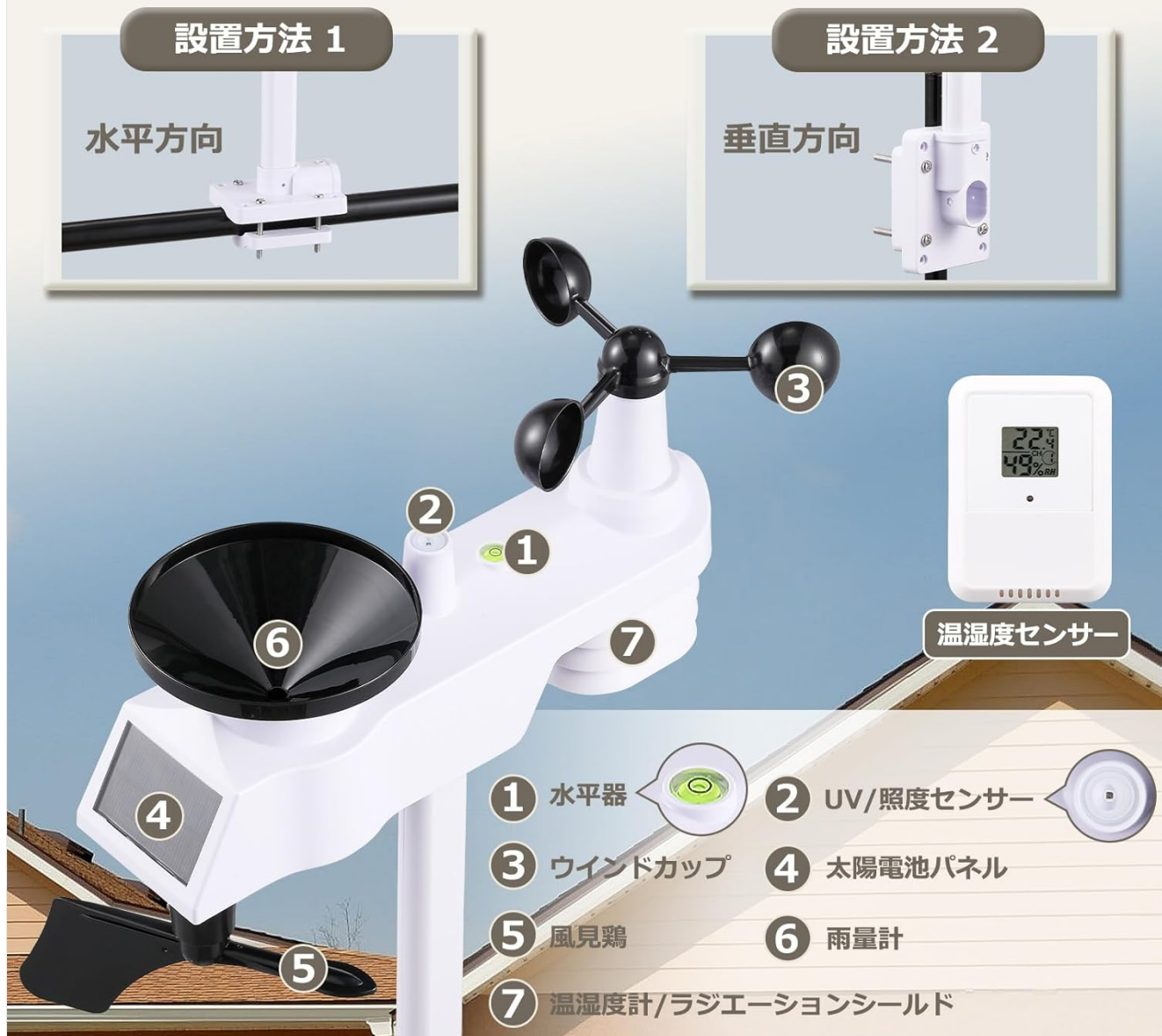
Figure 4.2: Outdoor Sensor Installation. This image details the outdoor sensor unit, showing its components (level, UV/illuminance sensor, wind cups, solar panel, wind vane, rain gauge, thermo-hygrometer/radiation shield) and two installation methods: horizontal and vertical mounting.
