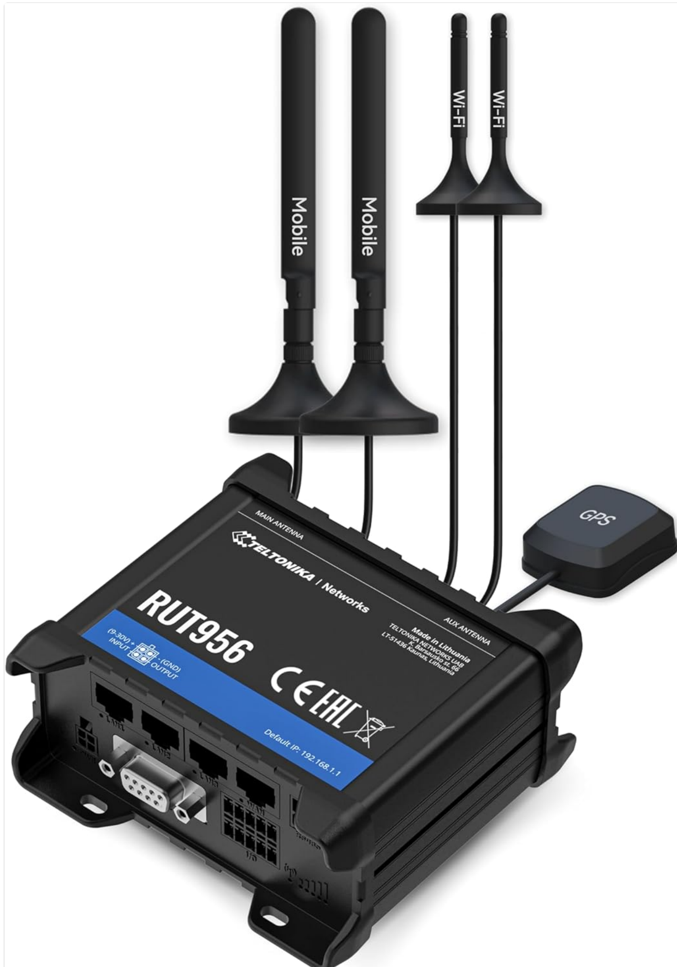
Figure 1: Teltonika RUT956 Industrial Cellular Router with connected antennas.
