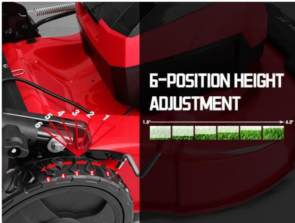
Image 5.2: The 6-position cutting height adjustment mechanism.
