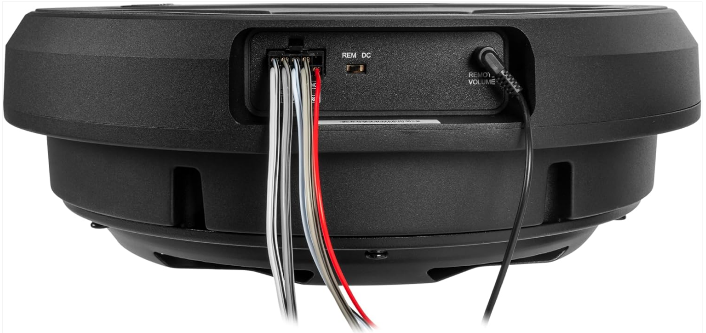
Image: Close-up of the wiring harness input side of the subwoofer, showing connections for signal input and remote turn-on.
