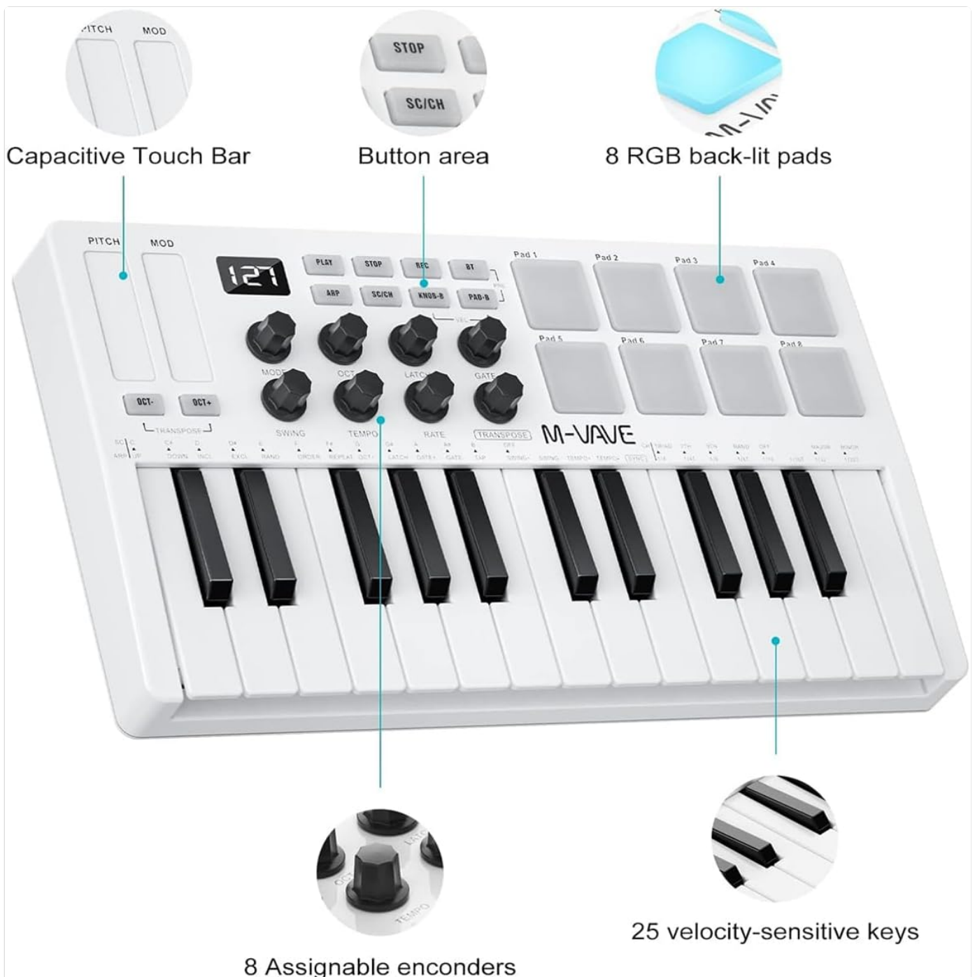
Figure 2.2: M-VAVE SMK-25 MIDI Controller with key components labeled.
