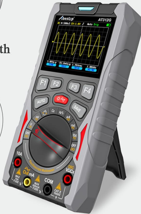
Figure 2.4: Additional features include a soft rubber sheath for protection, an audible beep alarm, and an integrated kickstand for hands-free operation.
