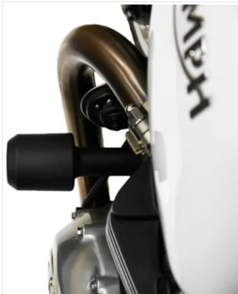
Figure 3.4: Frontal view of the frame slider installed, showing its alignment with the engine components.
