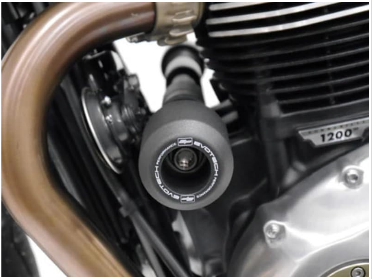
Figure 3.4: Frontal view of the frame slider installed, showing its alignment with the engine components.
