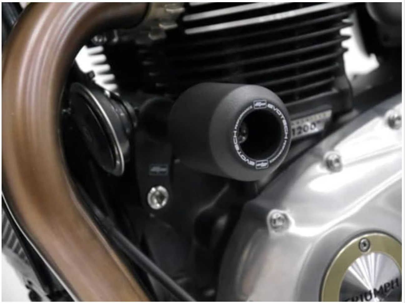
Figure 3.1: Close-up view of the frame slider installed near the motorcycle engine.
