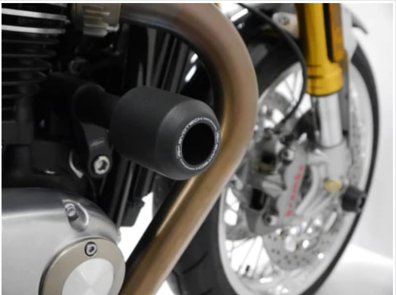
Figure 3.1: Close-up view of the frame slider installed near the motorcycle engine.
